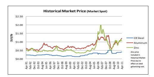
Steel costs less than aluminum on a \$/lb basis, but aluminum is approximately 1/3 the weight of steel. Using aluminum extrusions for the frame structure provides cost and performance benefits which far outstrip the pure material cost differences.
